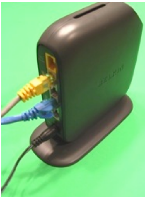
Figure 3 - Rear angle view of router showing the following connections from top to bottom (network [to camera base], network [to laptop computer], power)
