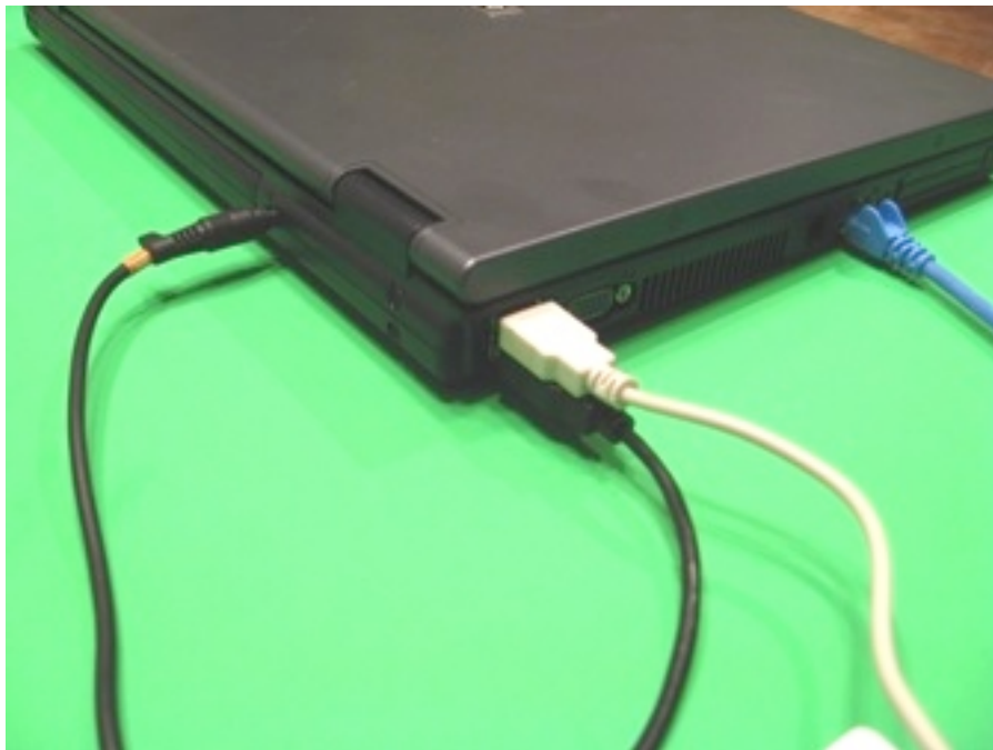
Figure 2 - Angle view of laptop showing the following connections from left to right (power, USB [bottom], optional USB for mouse extension cable [top], network)
