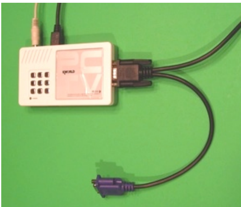
Figure 4 - Top view of PC 2 TV showing the following connections from top clockwise (power, SVideo, monitor [note that the black connector is used - not the blue])
