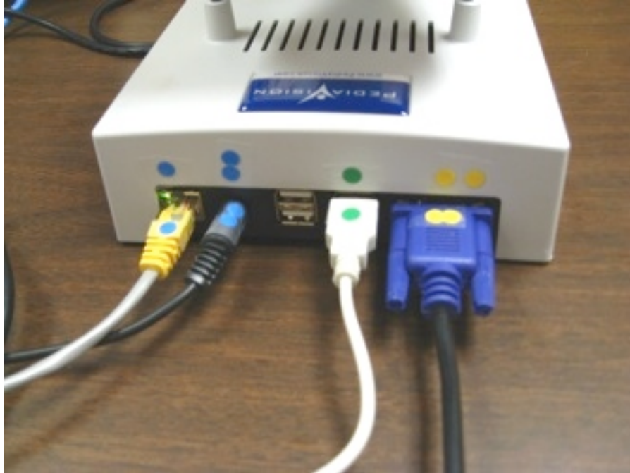
Figure 1 - Rearview of PlusOptiX Camera (base) showing the following connections from left to right (network, power, USB, monitor)
